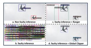
Figure 2: Visual example of faulty inferences on CoCo trained DINO-DETR model due to bit-flips caused by the soft errors.
