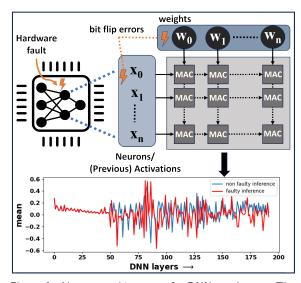
**Figure 1:** Abstract architecture of a DNN accelerator. The upper figure illustrates potential soft errors resulting in bit flips within neurons or weights at specific layers of the DNN model. The lower figure displays the mean values of layers in non-faulty inferences compared to faulty inference values when a bit-flip error is injected at the 50th layer of a transformer model DINO-DETR.
