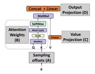
Figure 8: Individual components of Encoders and Decoders (Attention Blocks)
