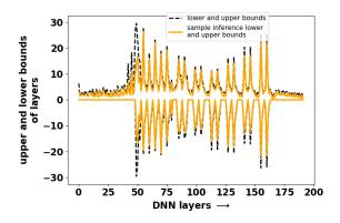
Figure 4: Lower and upper bounds for range restrictions, encompassing activation layers and linear layers within the self-attention blocks of the DINO-DETR model, are defined by the Global Clipper technique.
