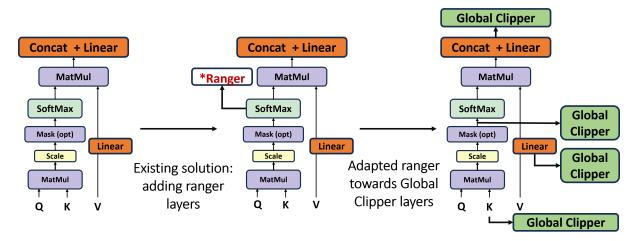
Figure 3: Integrating Global Clipper layers into transformer-based object detection models' self-attention blocks. \*Ranger layers are recommended to be added to activation functions, usually at ReLU layers, not SoftMax.
