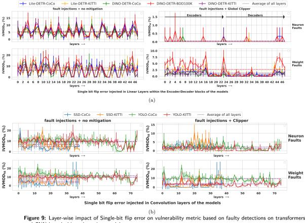
Figure 9: Layer-wise impact of Single-bit flip error on vulnerability metric based on faulty detections on transformers and CNN-based object detection models.
