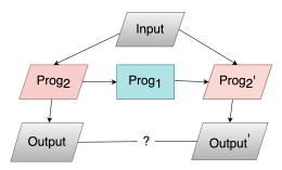
**Figure 1:** Traditional refactoring.  $Prog_1$  is the refactoring.  $Prog_2$  and  $Prog_2'$  are programs to be refactored and the refactored program, respectively. *Output* and *Output'* are the outputs of  $Prog_2$  and  $Prog_2'$ , respectively, given *Input*. Assume  $Prog_2 \neq Prog_2'$ .
