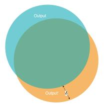
**Figure 3:**  $|Output'| \setminus |Output|$ . Output and Output' are supervised classification tasks' labels from the original and refactored models, respectively.  $|\delta| = |Output' \setminus Output|$ .
