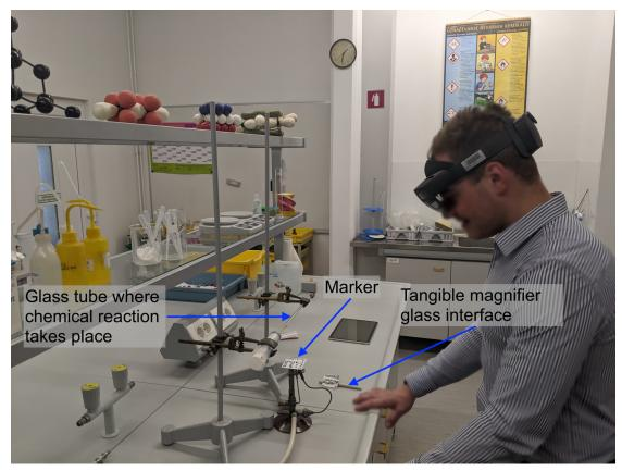
**Figure 1:** Laboratory setup in which the training is deployed. The observable phenomena occurs within the glass tube. The figure also shows a MARKER, which is used for positioning the visualisation and the TANGIBLE MAGNIFYING GLASS INTERFACE used to manipulate the VIRTUAL MAGNIFYING GLASS.
