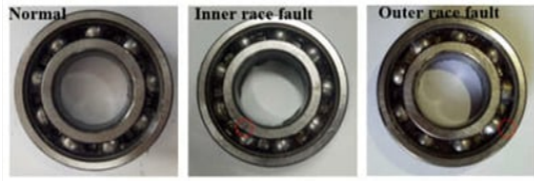
Figure 2: Typical fault cases introduced in the inner and outer races of the ball bearings.
