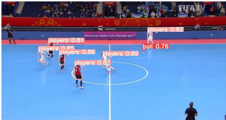
Figure 9: The results obtained using the proposed model, which detects players in futsal videos by knee, neck, and elbow parts of the body
