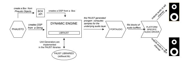
Figure 1: Overview of Phausto library and the embedded Faust dynamic engine.
