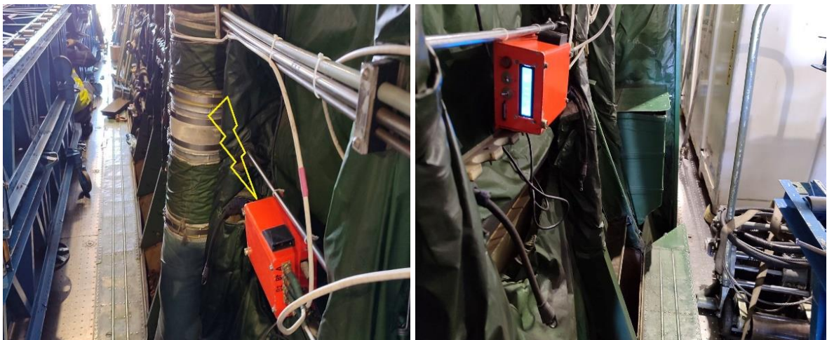
Figure 4: Computer IP-5 (Data acquisition, conversion, recording file on the SD card in *.txt format and transfer data via ethernet to the laptop).
