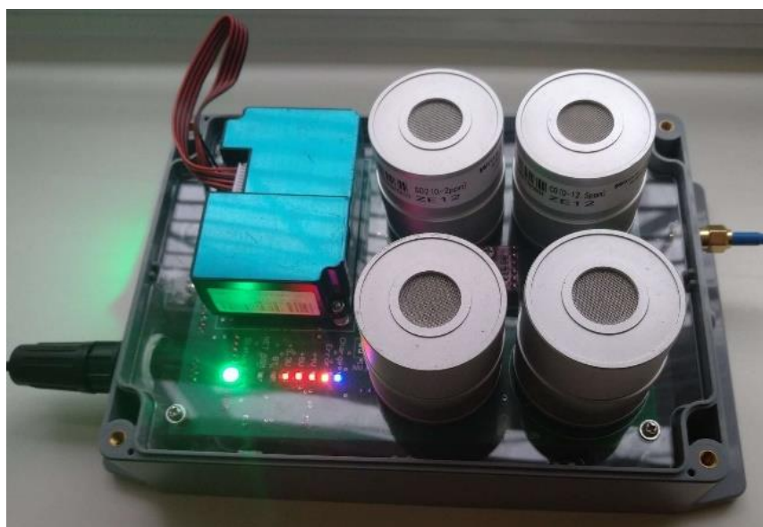
Figure 4: Monitoring station with ZE12 series electrochemical sensors.
