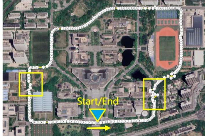
Figure 3: Description of kinematic experimental scenarios and trajectory of method A. The yellow boxes denote areas with severe obstruction.
