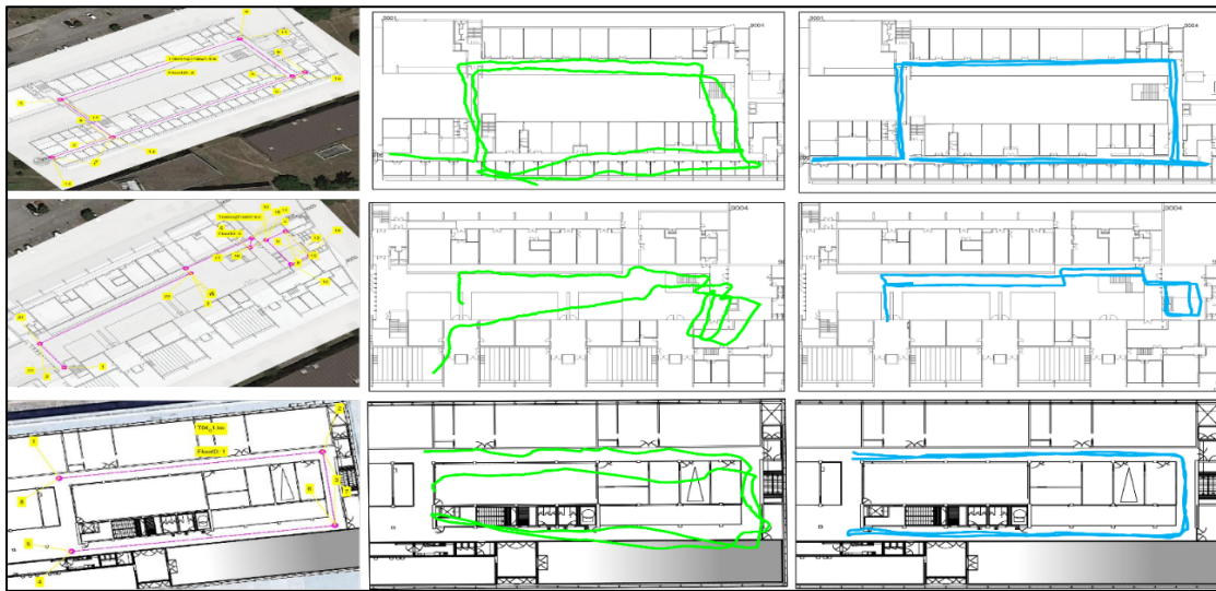
Figure 10. Three reconstructed paths and three columns are baselines, PDR result, and reconstructed path. *Note: All floor plans are showing the effect and were not used in the experiment.
