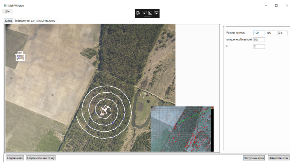
Figure 5: Simulating the flight of the UAV along the Archimedean spiral to find the position.
