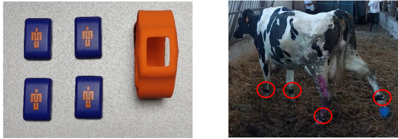
Figure 1: The Vicor Blue Trident IMU sensors (left) and their attachment to the cow's legs (right)
