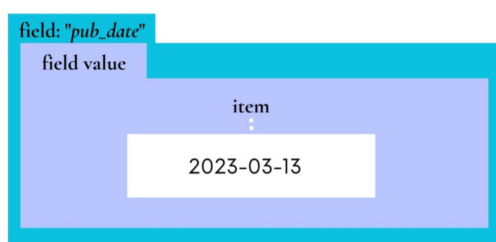
Figure 2: The abstract representation of the internal structure of the table cell containing the data for the publication date of a bibliography resource (see Table 1). The cell contains only one item, which corresponds to the value of the publication date. The publication date field always has a value containing a single item.
