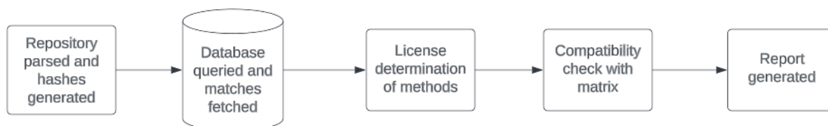
Figure 1: License violation detection flow
