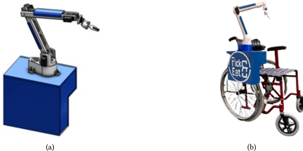
Figure 6: Wheelchair mounted robotic arm: a) proposed concept; b) a prototype.
