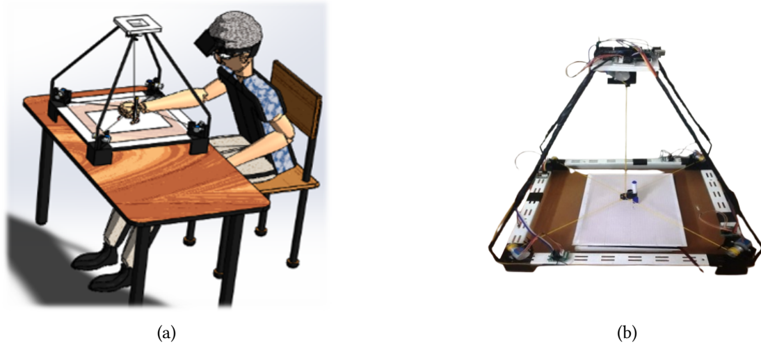
Figure 7: Pyramidal cable driven robot: (a) concept; (b) prototype at UNICAL.
