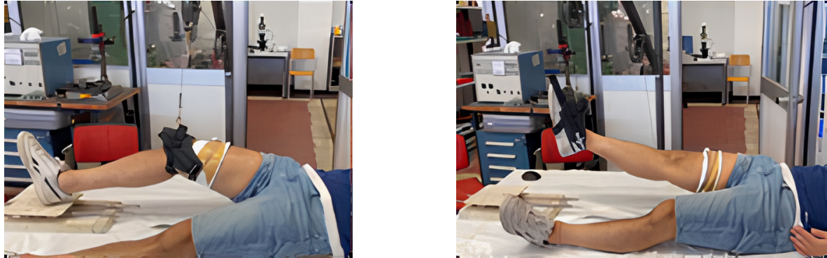
Figure 4: A prototype of a cable-driven lower limb device at UNICAL.
