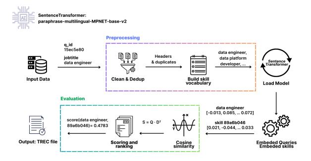
Figure 1: Diagram of the System's Pipeline
