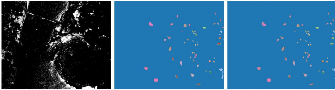
Figure 8: Prediction maps for KSC dataset (5% training ratio). Figure shows spectral band, ground truth, and classification result
