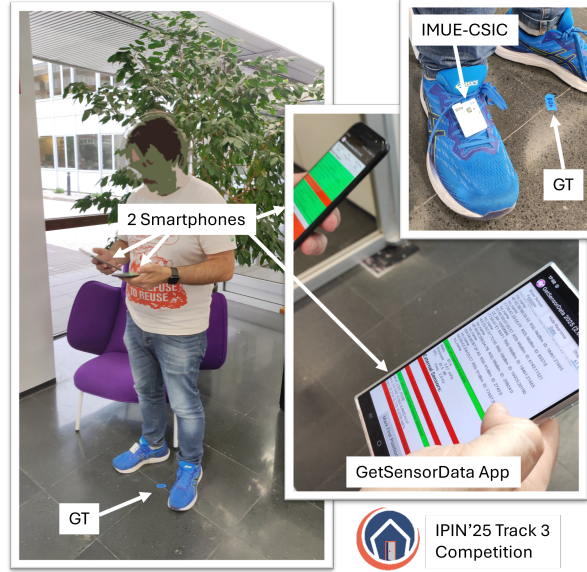
Figure 1: Illustration of the data collection setup during the IPIN'25 Competition (Track 3), showing the two smartphones running the GetSensorData App (release June 2025), the GT marks placed on the floor, and the foot-mounted IMU (model IMUE-CSIC).
