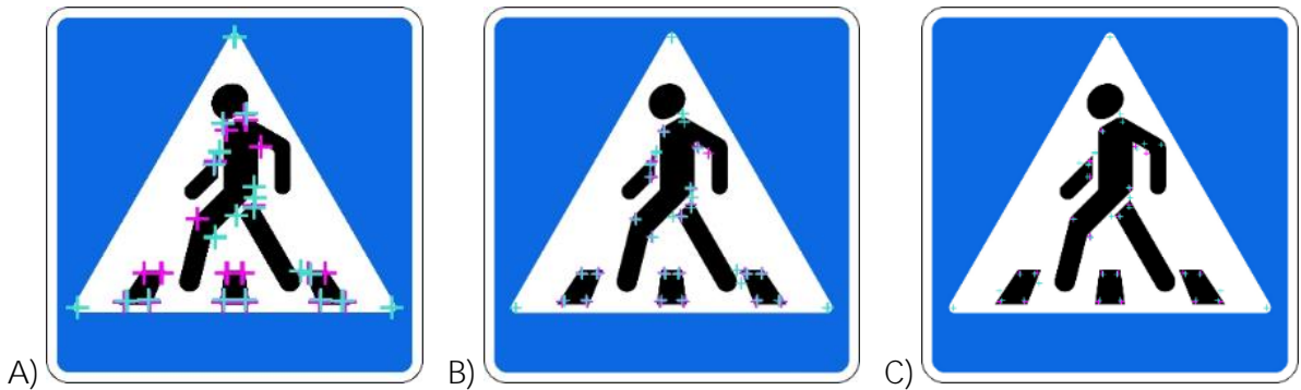
Figure 3: SIFT octaves with SIFT/BRISK-keypoints on the traffic sign “Crosswalk left” (images are not scaled according to the SIFT octaves’ sizes): octave 340×340 pixels (A), octave 680×680 pixels (B), octave 1360×1360 pixels (C).
