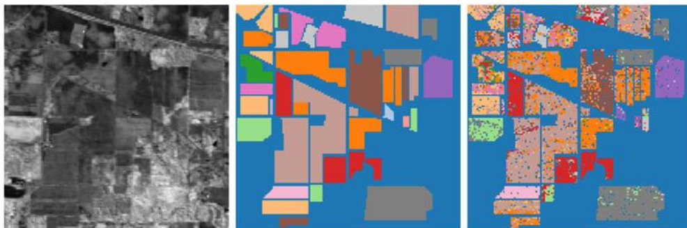
Figure 3: Prediction map for the Indian Pines dataset (OA = 68.96%). From left to right: original spectral channel, ground truth (GT), classification result.
