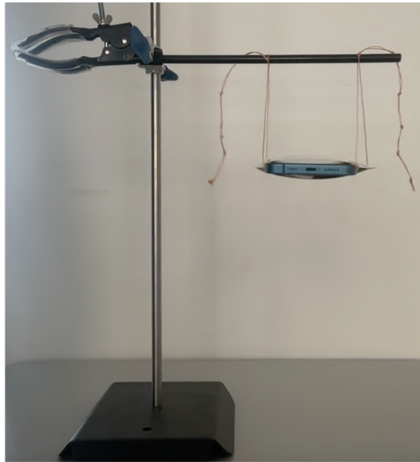
Figure 5: This setup was used to measure the time period of a pendulum and find acceleration due to gravity. To accurately measure the time period, the windows were closed to avoid interference.
