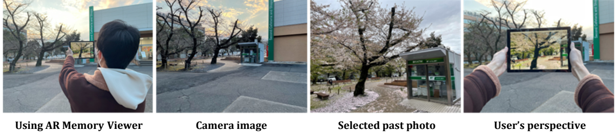
Figure 1: AR Memory Viewer allows a user to view past scenes through the screen of a user's mobile device. Feature point matching is performed between the camera image and a past photo, and the past photo is aligned with the camera image and displayed as an AR superimposition on the screen of the mobile device.
