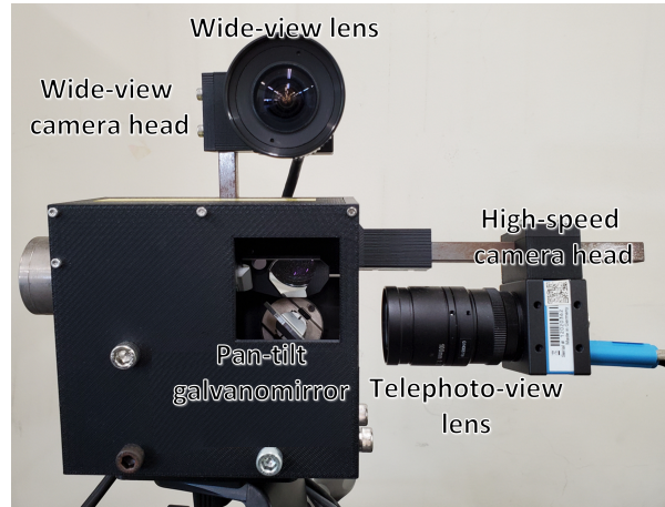
Figure 2: Camera module with an ultrafast pan-tilt camera and a wide-field camera. The galvano mirror steers the magnified camera's line of sight at high speed.
