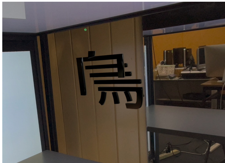
Figure 4: Perspective view of three-dimensional font object of the Chinese character “Bird,” featuring stroke-order-following depth extrusion and a glossy appearance in UD Shin-Gothic font.
