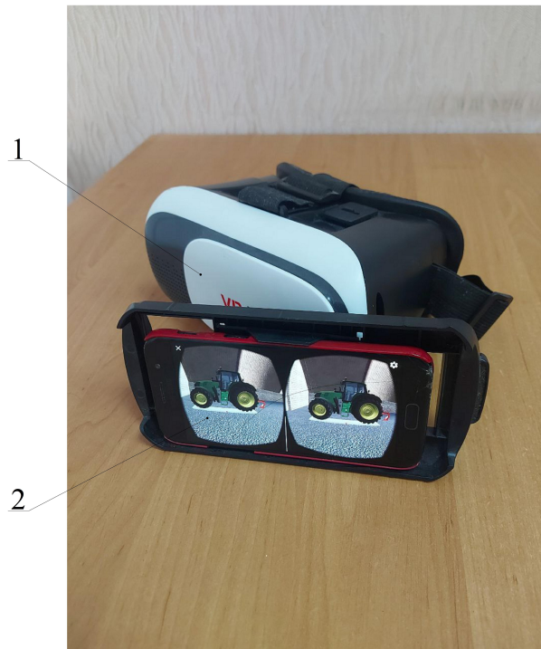
Figure 1: Training equipment such as Google Cardboard: 1 - VR-glasses; 2 - clamp and phone with the developed application.
