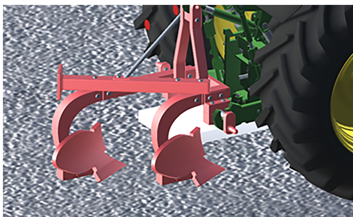
Figure 6: Adjusting the working width of the plough.
