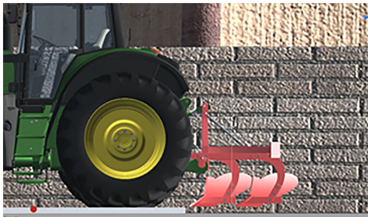
Figure 4: Horizontal levelling of the plough in the longitudinal direction.
