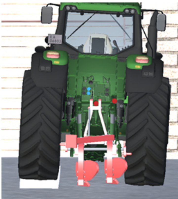
Figure 5: Horizontal levelling of the plough in the transverse direction.
