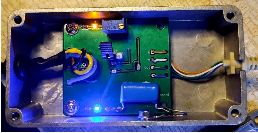
Figure 3: Specialized amplifier board with AD8221.
