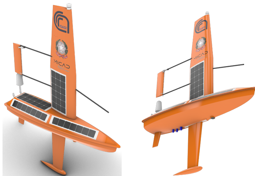
Figure 1: The I-Boat autonomous sailboat with navigational and environmental sensors.
