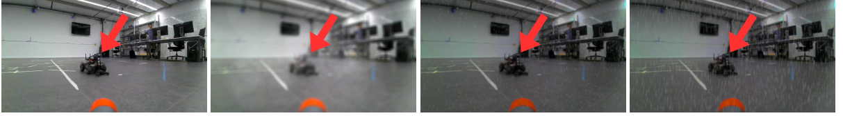
Figure 2: Robot as captured by the camera, along with simulated exogenous factors. In order from left to right: original, fog, low rain, strong rain.
