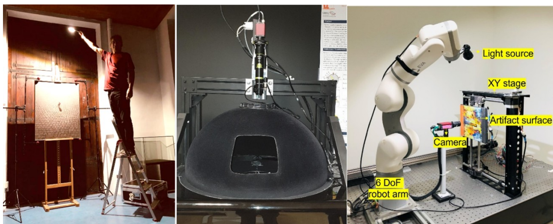
Figure 2: some examples of RTI implementation. Handhel (left), Dome-based (middle) and Robotic-arm based ((right)
