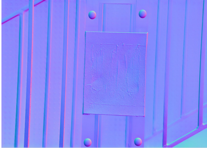
Figure 11: normal map derived from acquired RTI data using the proposed setup.
