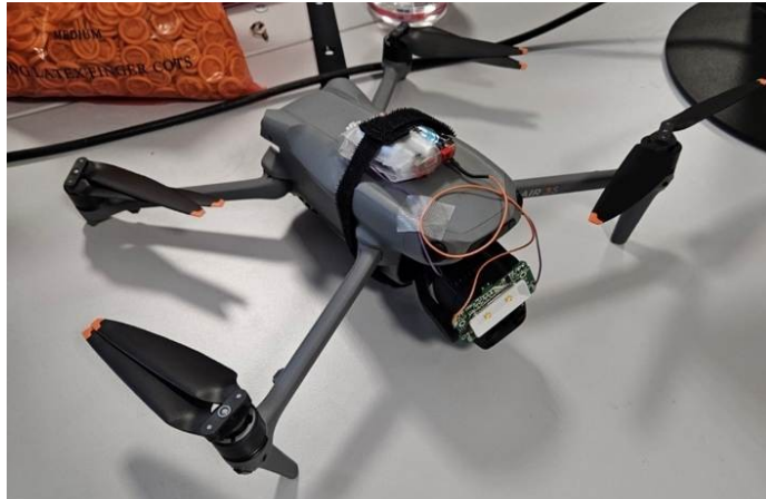
Figure 5: The drone, equipped with the light source
