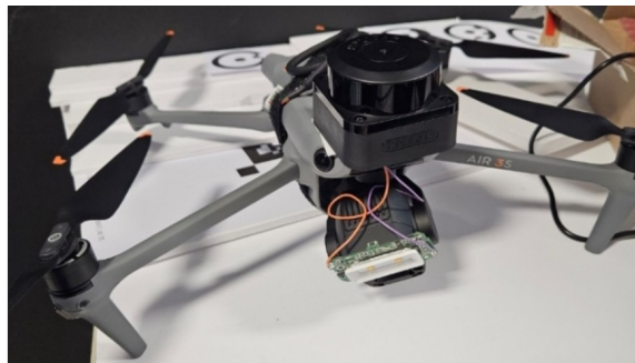
Figure 12: DJI Air3S, equipped with LiDAR and ESP32, allows it to map its environment from the camera stream.
