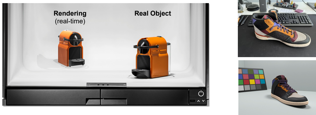
Figure 5: AxF enabling visual digital twins of products' material appearance. Left: comparing digital twin and physical product in a calibrated viewing booth. Right: using digital material twins to achieve novel product visualizations (below).
