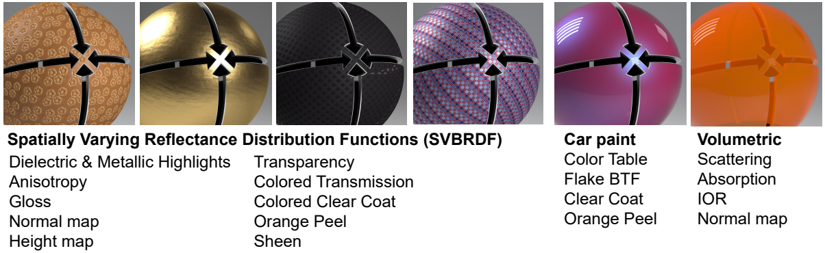
Figure 4: The main appearance rendering representations and their components as specified in AxF.
