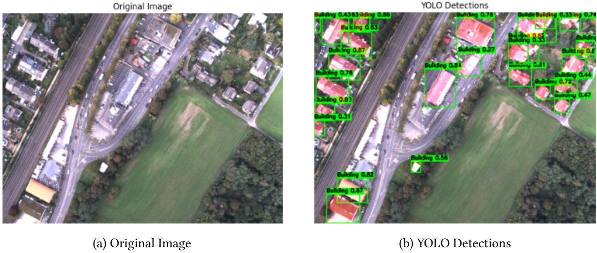
Figure 6: An example of building segmentation on an image from the VPAIR dataset.
