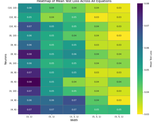
(b) Test Loss Heatmap for HybridKAN
