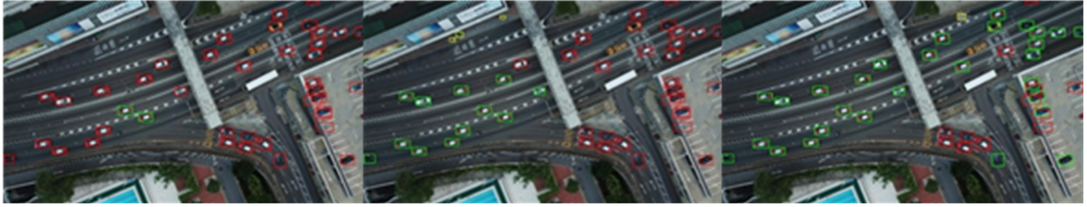
Figure 8: Object detection results on a test image for networks trained on synthetic data from the first, second, and third iterations (left to right). Legend: TP (green box), FP (yellow box), FN (red box).
