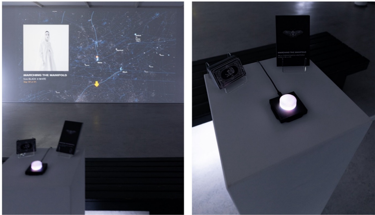
Figure 5: The 3D-printed physical controller on a podium. The final design incorporates a single, push-enabled turning knob, driven by an RP2040-based development board. The projection of the web interface is situated in the background on the wall.
