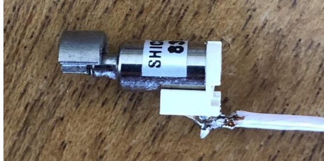
Figure 7: View of the used vibration motor.
