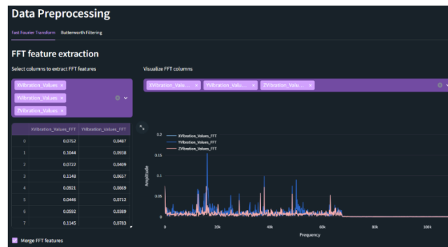
Figure 3. Vibration FFT feature extraction through i4Q DIT
