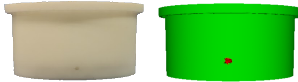
Figure 2: Highlighted in red detected surface defect spot on a plastic coffee capsule.
