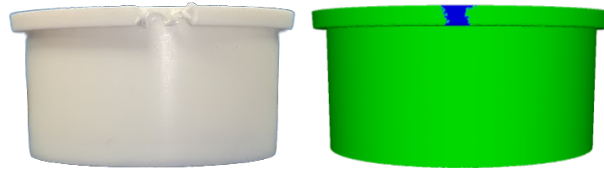
Figure 1: Highlighted in blue detected volumetric missing volume on a defective plastic coffee capsule.
