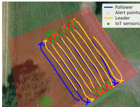
Figure 6: IoT sensor proximity query result, showing robot positions (red) within the sensor range during intervals where the sensor reading exceeded the defined threshold.
