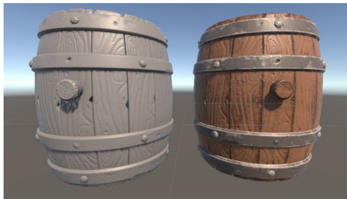
Figure 3: Comparison of high-polygon version and low-polygon version with baked textures.
