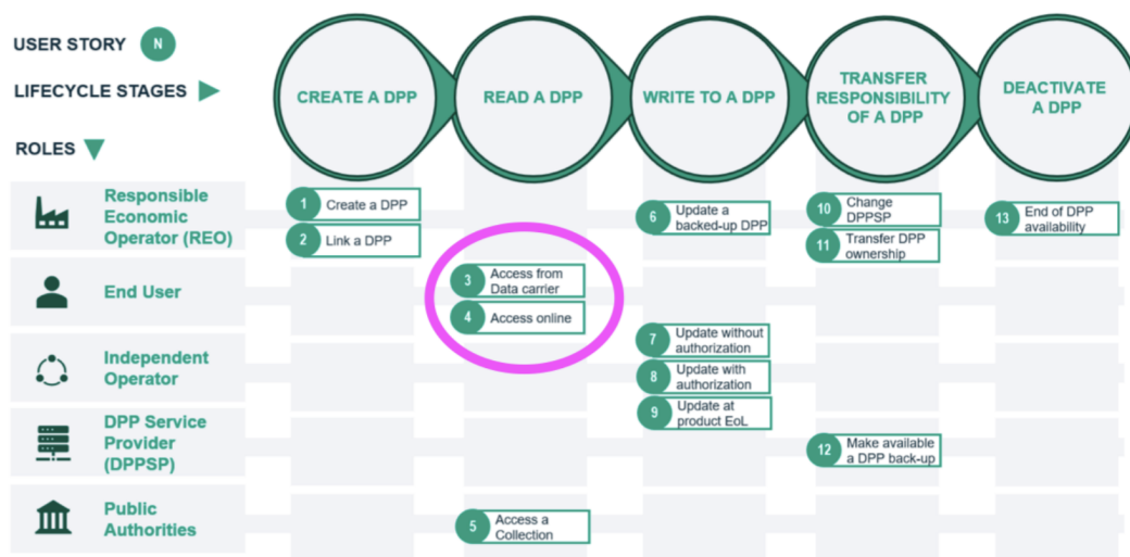
Figure 1: Figure 6 from ‘User Stories’ document for the European DPP system, i.e., interactions between the DPP system and its intended users.[12]. Purple highlight by me.
