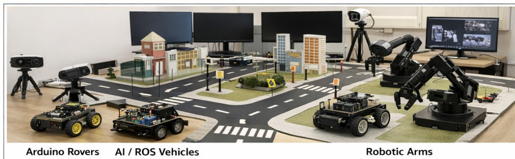
Figure 2: Physical implementation of the Smart City robotics educational laboratory with mobile robots, robotic manipulators, camera-based remote access, and integration with a cloud-based virtual learning environment
