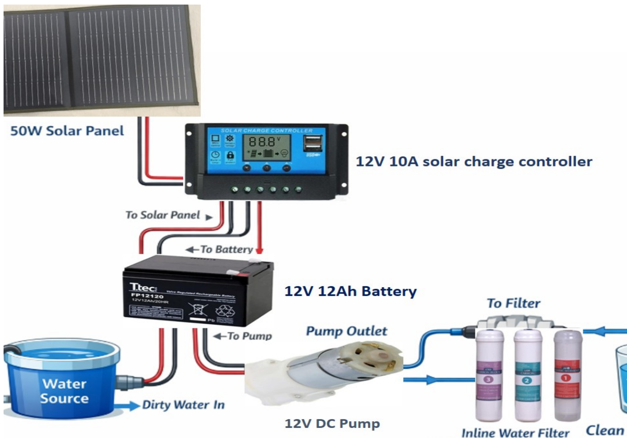
Figure 1: Solar-powered portable water purification prototype developed within the SunGel study.
