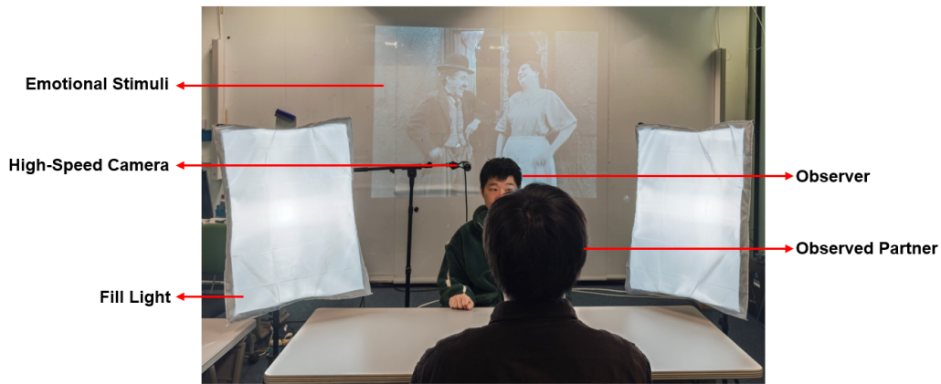
Figure 4: Recording environment for first-person perspective video.
