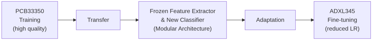
Figure 3: Transfer learning process PCB33350 → ADXL345
