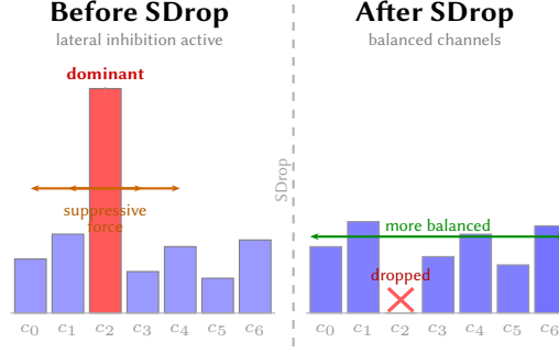
(a) Lateral inhibition concept. Left: dominant channel c_2 (red) suppresses neighbors. Right: after SDrop drops c_2 , remaining channels are more balanced.
