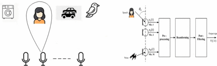
Fig. 2. Extracting the desired target speaker by using microphone array. Fig. 3. The scheme of microphone array signal processing.
