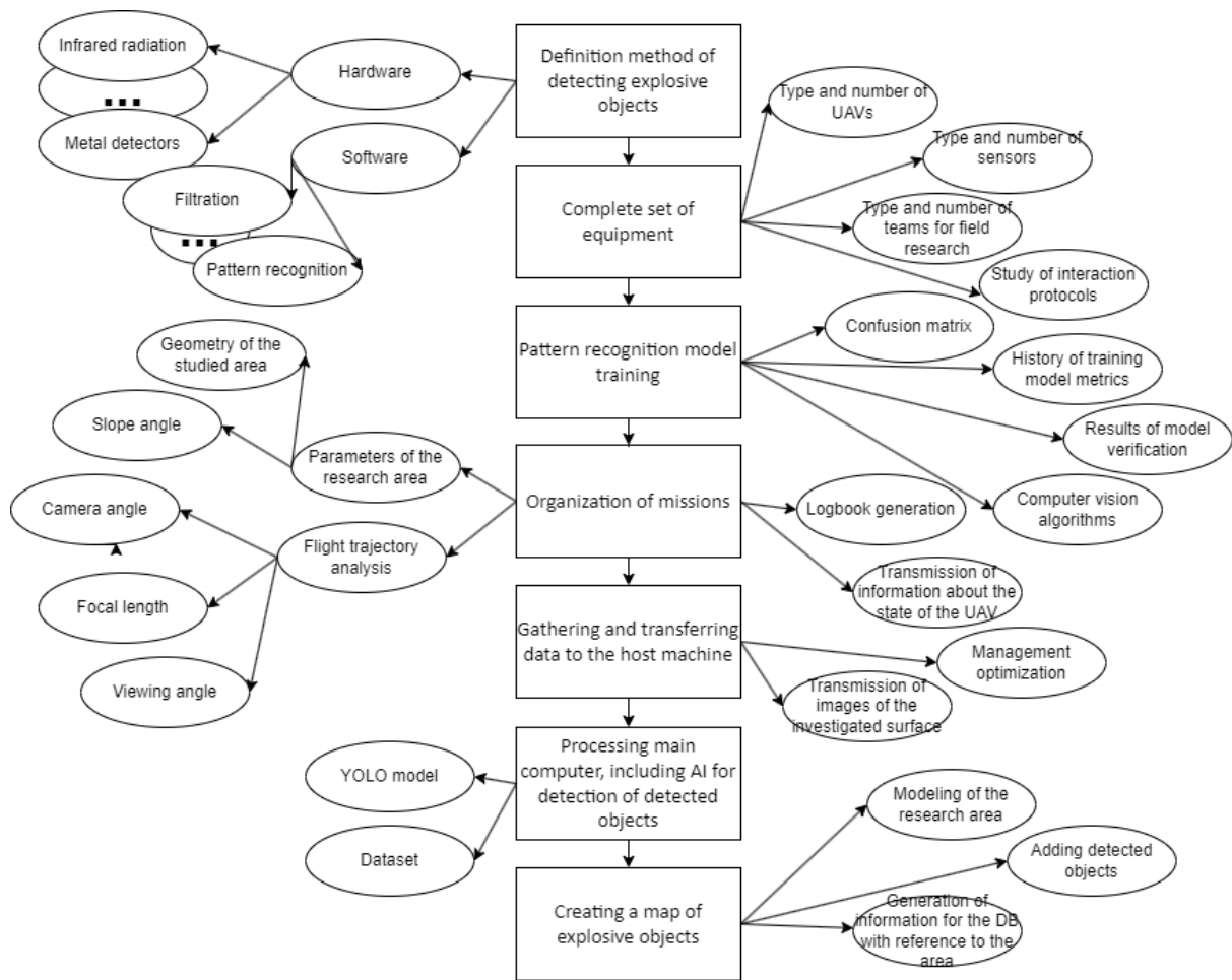
Figure 3: Stages of organization of the system of detection, detection, accounting and visualization of explosive objects.
