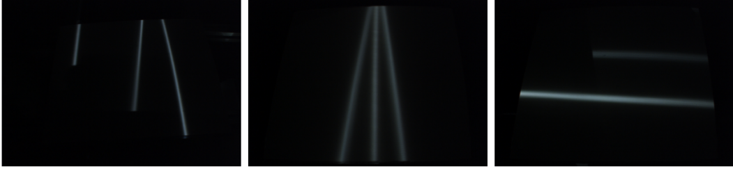
Figure 5: Captured image showing that a single projected line appears as multiple lines on the stage after reflection by multiple mirrors.
