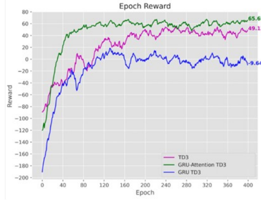
Figure 11: Comparison of moving average epoch reward for TD3, GRU-TD3 and GRU-Attention TD3 networks
