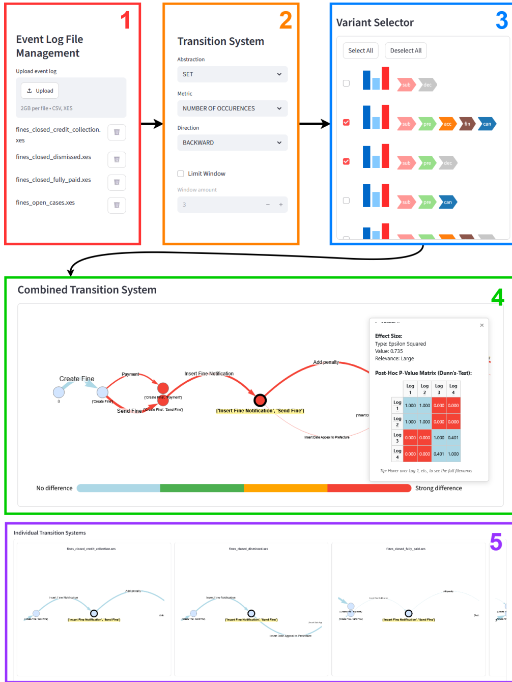
Figure 1: The workflow of the tool: (1, red) upload logs → (2, orange) choose settings → (3, yellow) select variants → (4, green) analyze the combined transition system, and (5, purple) individual transition systems.
